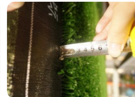
Step5: Quality control (pile)
